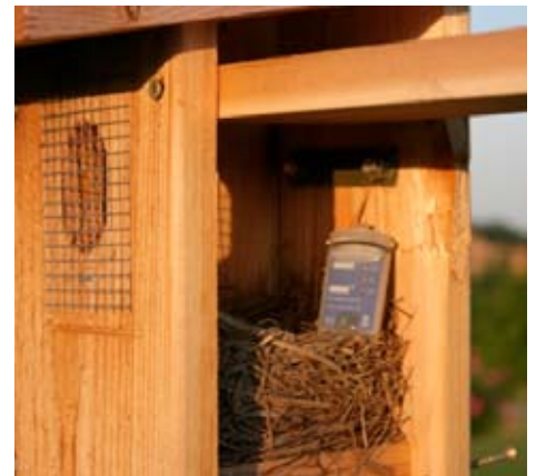
Figure 3. HOBO Pendant hourly temperature logger in nest.
