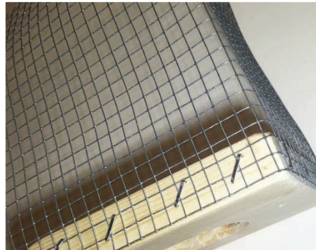
The wood block is optional. You can attach the wire directly to the front of the box with several screws but the block of wood makes a sturdier guard.
