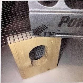
The wood block is optional. You can attach the wire directly to the front of the box with several screws but the block of wood makes a sturdier guard.
