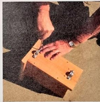
The wood block is optional. You can attach the wire directly to the front of the box with several screws but the block of wood makes a sturdier guard.
